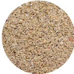
Coarse sand is rather large size and unequal forms with edges. It is suitable for structural construction work that requires stronger forces e.g. bridges, reinforced structure, footing, land, land slide prevention etc.
