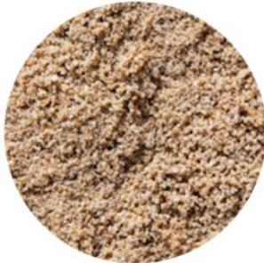
Fine granular or fine sand has the shape of round and solid grains. It is the cleanest among the other types of sand. It is suitable for plastering works that require fine texture and to be used at the golf course. It can also be used to produce light weight brick
