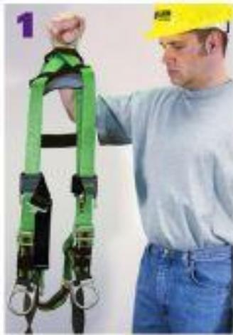
**1** Hold harness by back D-ring. Shake harness to allow all straps to fall in place.
