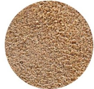
Fill sand is commonly used for leveling and or used together with sandbags that help prevent flood and road filling
